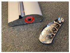
3. Insert the crank into the slot within the red circle and turn counterclockwise until the banner has been re-wound into the base. Replace the metal end of the panel base and follow set up instructions as normal.
